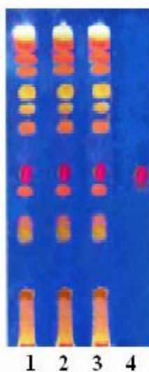
TLC profile of test solution of Bixa orellana seed. 1-3 : Test solution; 4 : Bixin standard.
