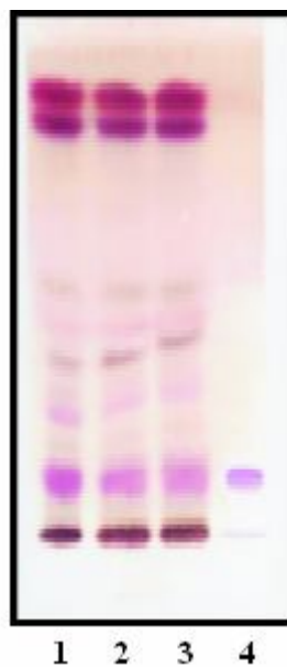
TLC profile of test solution II of Alstonia scholaris stem bark derivatized with anisaldehyde-sulphuric acid reagent. 1-3: Test solution II; 4: Echitamine standard.
