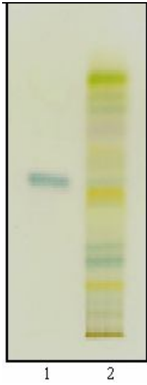
TLC profile of test solution of Taxus wallichiana needle extract. 1: Paclitaxel standard; 2: Test solution.
