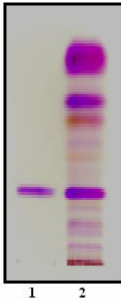
TLC profile of test solution of Mimusops elengi stem bark extract. 1: Lupeol standard; 2: Test solution.
